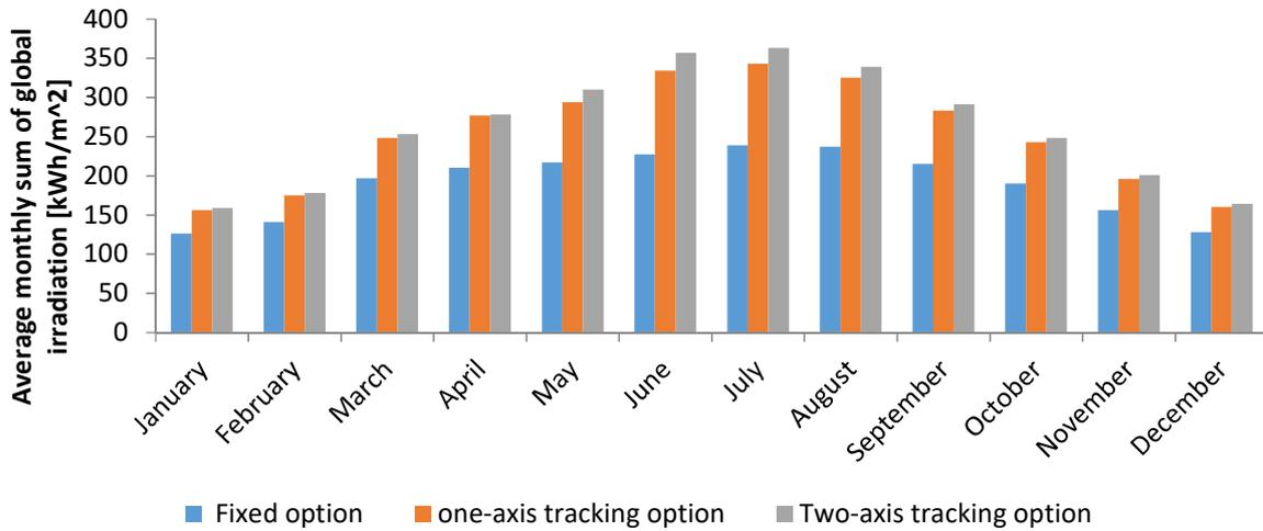
Figure 4. Monthly in-plane irradiation for Lefke at various mounting options
